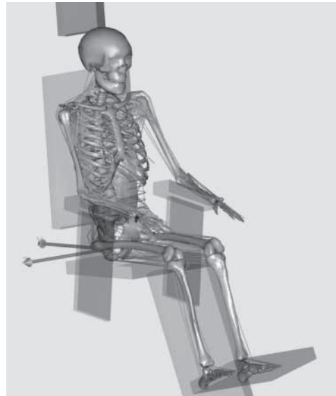
Figure 1 show the musculo-skeletal model developed in the AnyBody Modeling System
